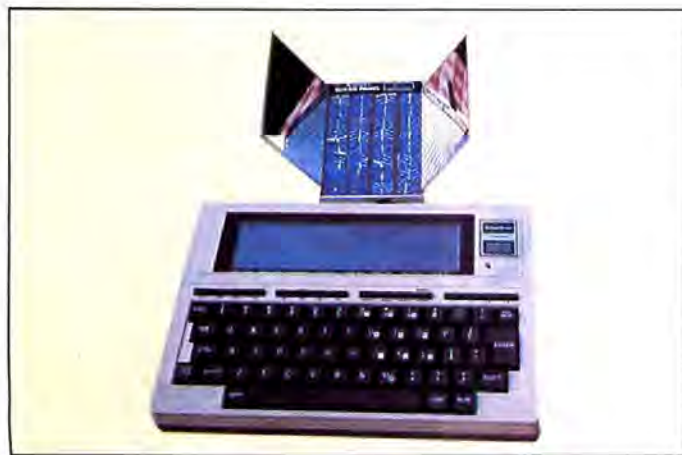
Photo 3. A solar power panel for the Model 100.
