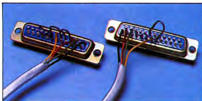
Photo 4. Pin connections for null modem RS-232 connectors.
