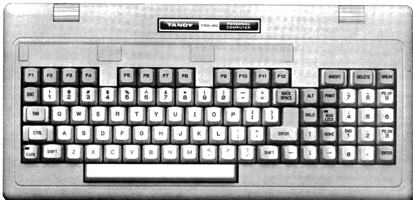
Photo 5. The Model 2000 keyboard. The non-number keys are tiered down the keyboard, but the numeric keypad keys lie flat.
