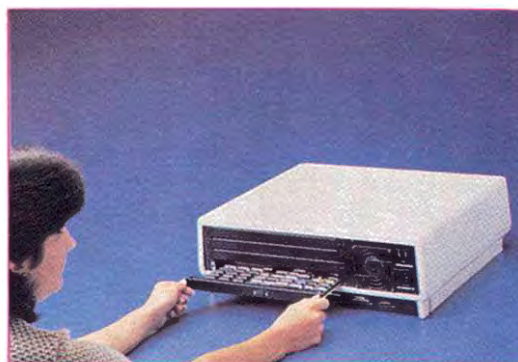
Photo 1. The Model 2000's expansion boards install easily. The board comes mounted on a tray; you slide the tray into an expansion slot at the back of the CPU case. Two lock buttons on either side of the tray hold the board in place.
