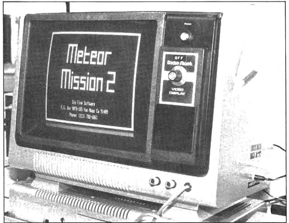
Photo 1. Completed installation. Notice the centered control knob directly below the Radio Shack logo; the black speaker grating for covering speaker holes; and the marked audio and power jacks on the casing's right side.
