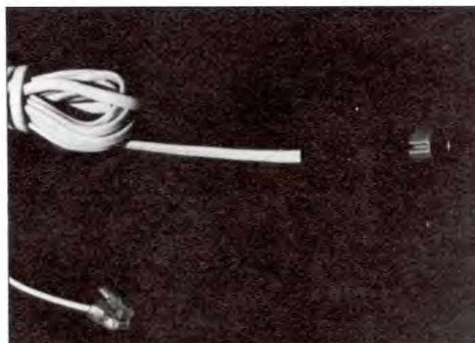
Photo 4. Completed modem cable.
