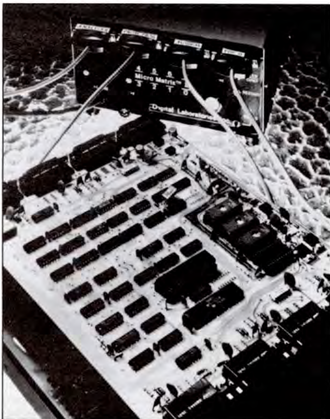
The Micro Matrix II: A software-controlled data switch that connects RS-232C, Current Loop, and TTL devices.
