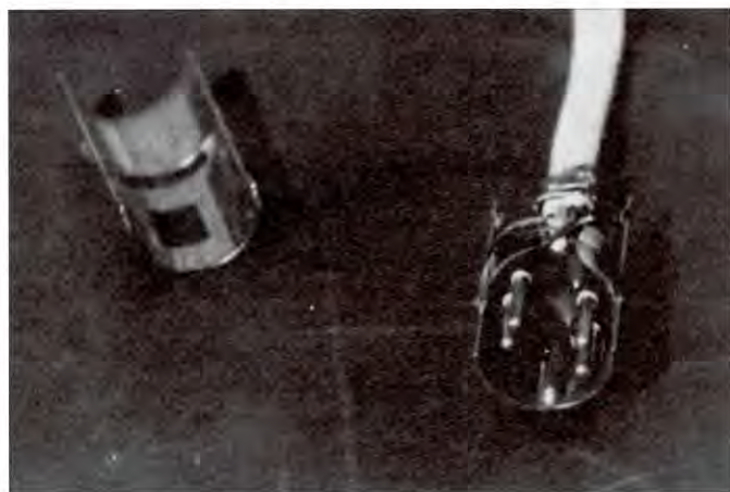
Photo 3. The red wire goes to pin 3, while the green wire goes to pin 7.
