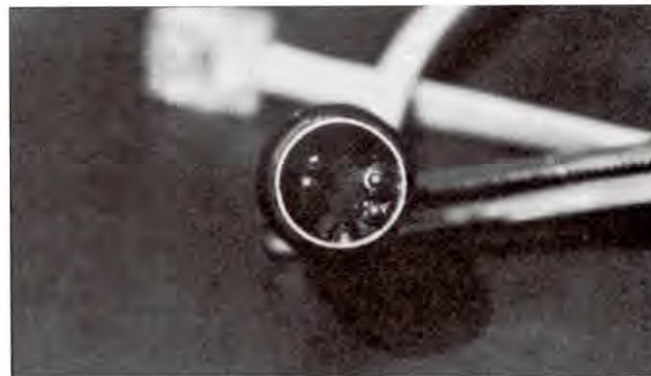
Photo 2. 5-pin DIN plug with new pin 7.
