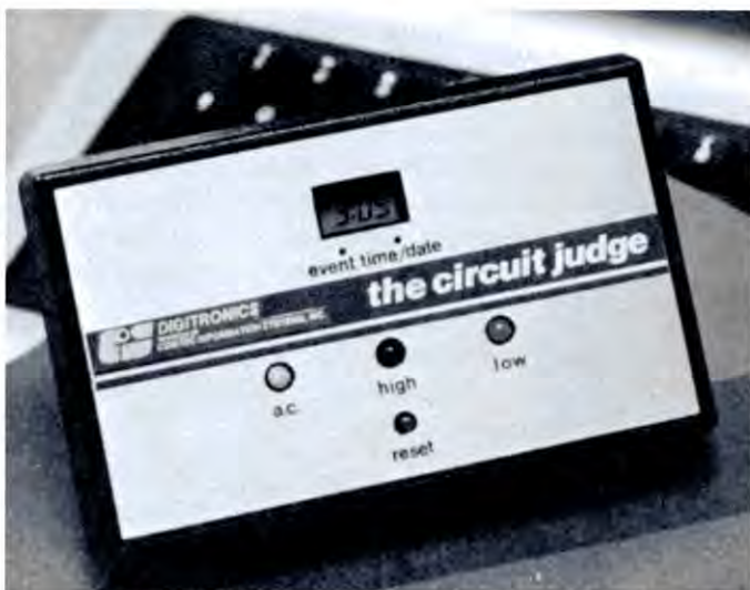
Know the time and date of a power failure with the Circuit Judge.
