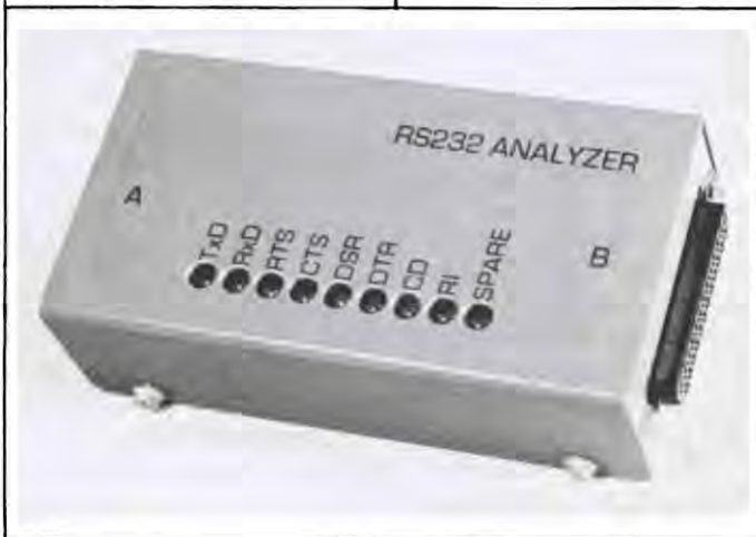
The RS-232 Analyzer: It monitors your RS-232 interface signals.
