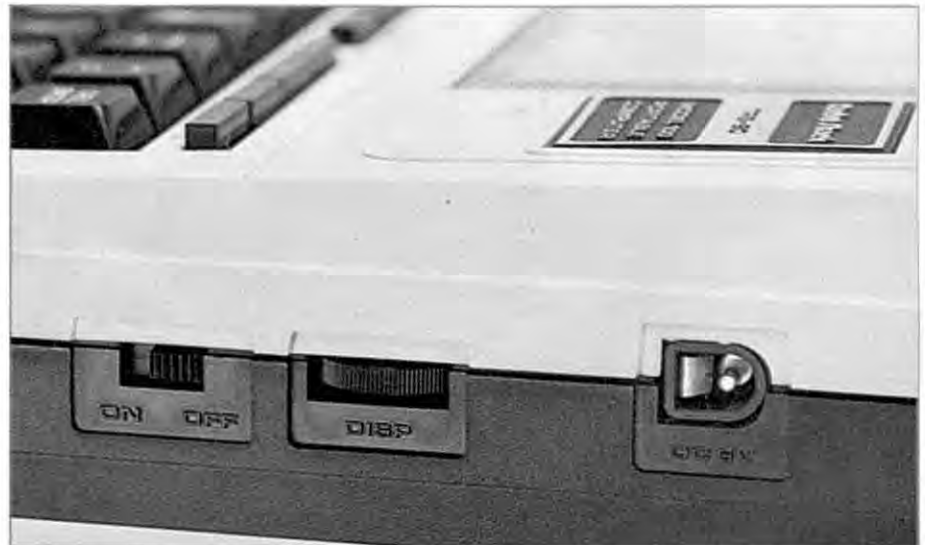
Photo 2. Right side of the Model 100 showing (from left to right) the on/off switch, display adjustment, and 6V dc power jack.
