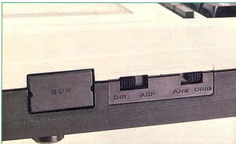
Photo 4. Left side of the Model 100 with (from left to right) the bar code reader port, a direct-connect/acoustic modem switch, and the answer/originate mode switch.
