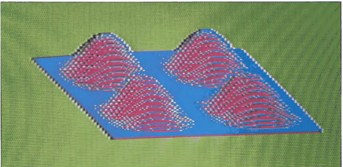
Photo 4. This photograph shows a three-dimensional view of eight sine waves. Four of the waves are in the horizontal direction and four are in the vertical direction. The end result is four "hills" on what appears to be a flat surface.
