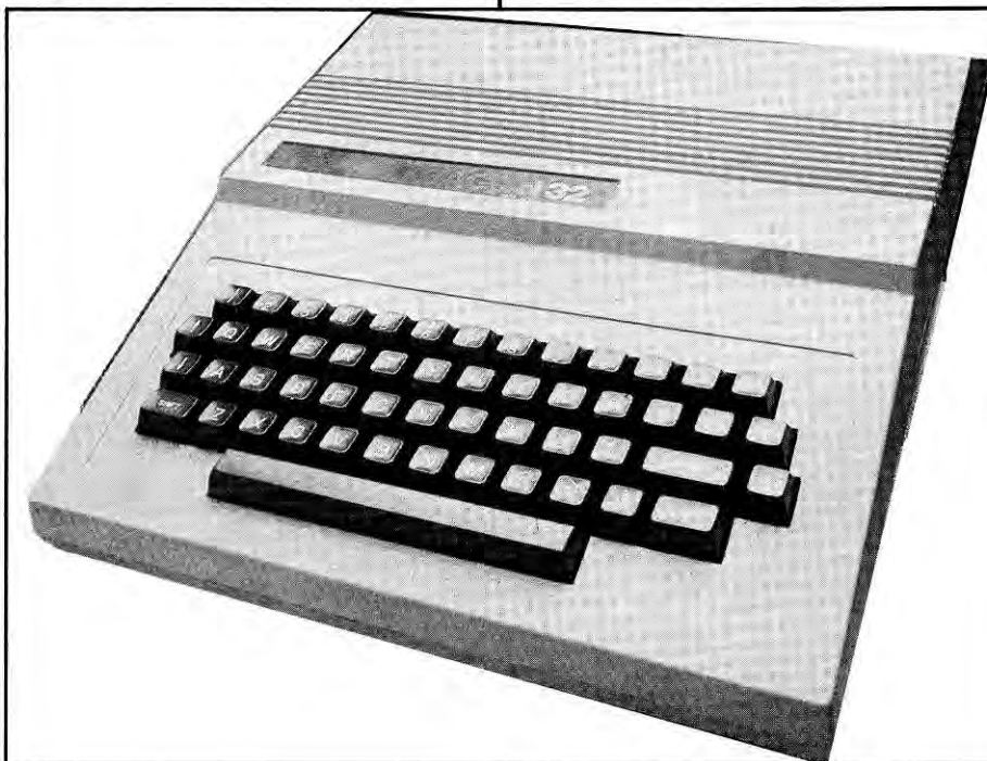
Tandy UK: 80 percent of the Color Computer's ROM packs will run on the Dragon 32.
