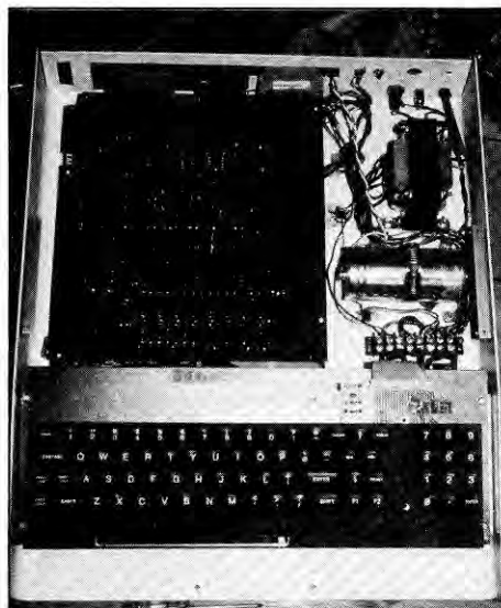
Photo 3. The expansion board is oriented upside down and bolted above the main CPU board. Off-size washers and close traces shorted out the system several times before I discovered the physical problem.
