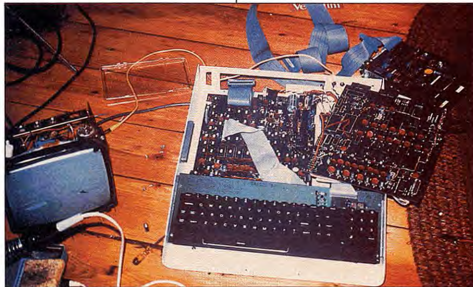
Photo 2. The LNW expansion board (at right), a monitor (at left), and a disk drive (back right) are all connected for testing. The keyboard is bolted in place and connected. This unit (the second of two built for this article) worked on the first try.
