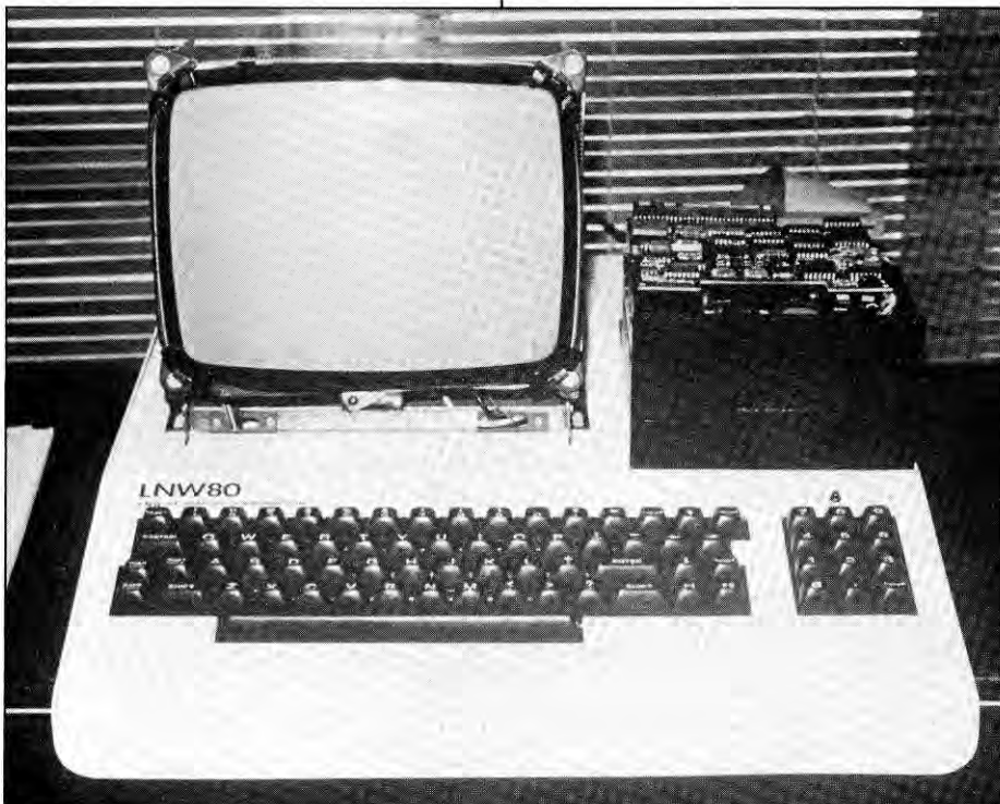
Photo 4. The finished LNW-80. The monitor and single drive are fastened to the case below with strips of foam tape, making a secure and transportable—though quite heavy—system.
