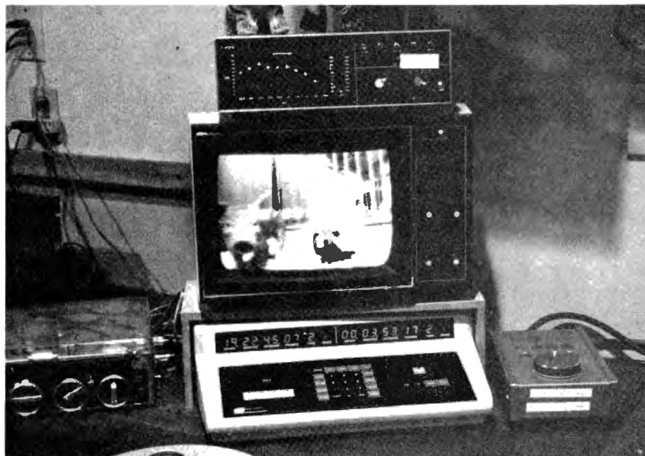
An editing computer in the author's studio. The three sets of numbers (two on the keyboard, one on the screen) are SMPTE code locations. The LED graphic display above the screen is a spectrum analyzer.
