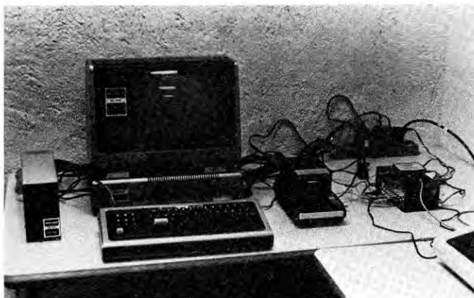
Photo 1. Master Computer: Model I 48K with single disk drive and Stringy Floppy.
