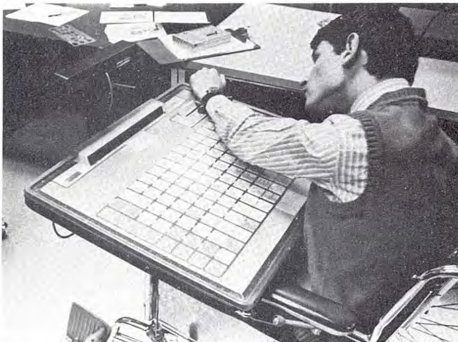
Photo 1. Joel Stevey uses a magnet strapped to his watch to select the components of his message.
