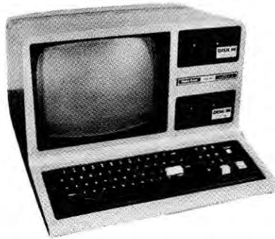
1 DISK III single drive assembly includes: one 40 track 5 1/4" double density drive, power supply, controller, mounting hardware, and applicable cables.
