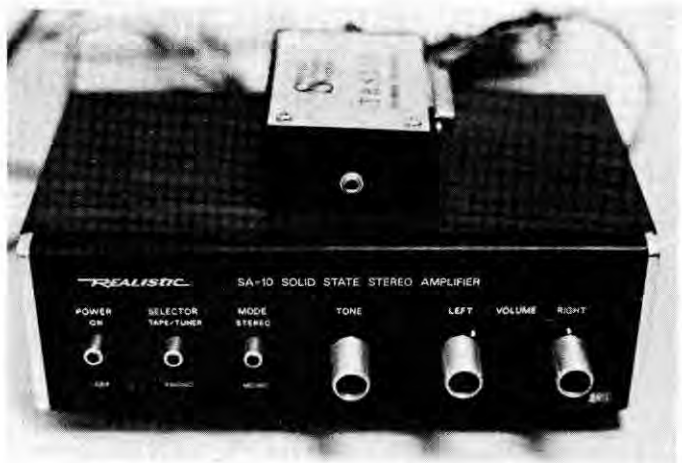
Photo 3. Front of amplifier Selector to tape/tuner: Mode—Stereo; Tone—Fully counter-clockwise; Left—Receive channel; Right—Send channel.
