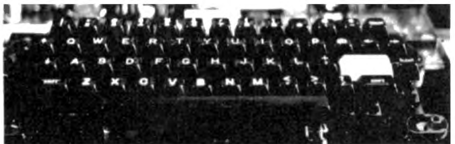
Photo 12. The modified keyboard installed in the Color Computer.
