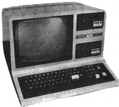
1 DISK III single drive assembly includes: one 40 track 5 1/4" double density drive, power supply, controller, mounting hardware, and applicable cables.
