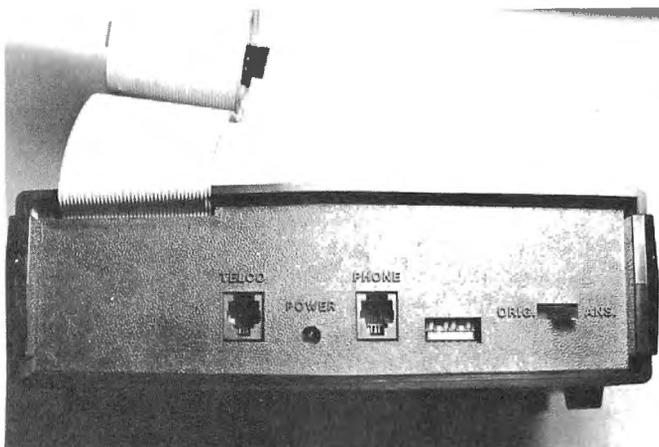
The back panel of the Lynx has telephone connections, user programming switches, and originate answer switch.
