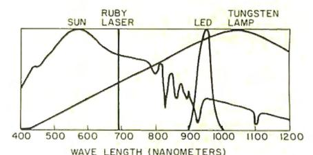
Fig. 5. The spectra of various light sources used in robotics experiments.
