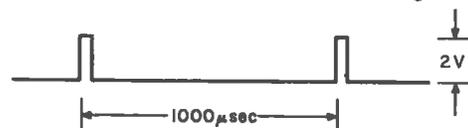
Fig. 1c. Wave-shaping Device Output
