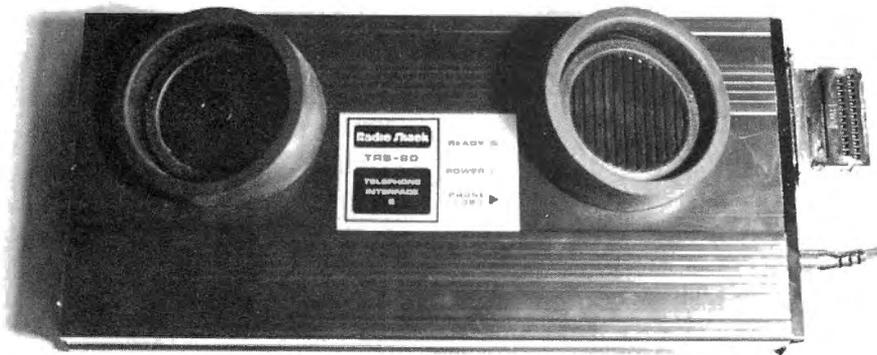
*The Telephone Interface II modem; telephone handset cradles in the rubber cups.*
