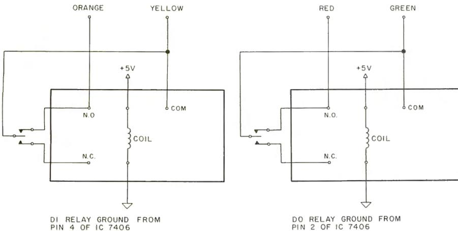
Fig. 4. Robot control relay connection schematic shows color coded relay outputs: D0 = 1 and D1 = 0 command translation; D0 = 1 and D1 = 1 command head rotation; D0 = 0 and D1 = 0 give no motion.
