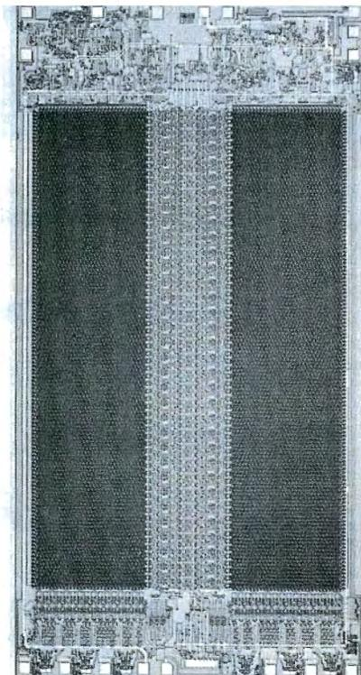
Fig. 1. Mostek Co. Memory Circuit Chip (*Scientific American*, 1977).
