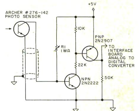
Fig. 2. Optical signal conditioner converts light input into a voltage proportional output.
