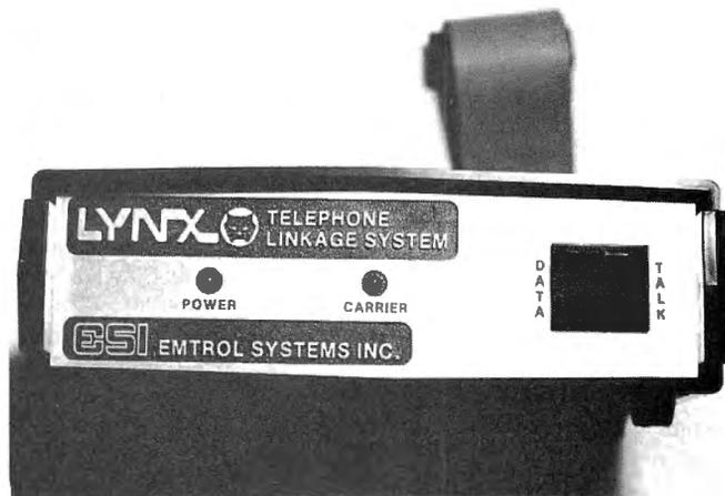
The front panel of the Lynx indicates carrier, and has voice data switch.
