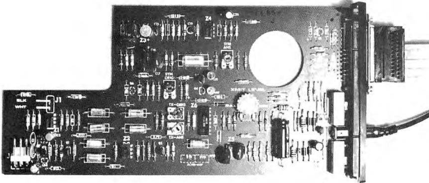
*Inside the Telephone Interface II: holes and slot are for microphone and speaker, disconnected in this photo.*
