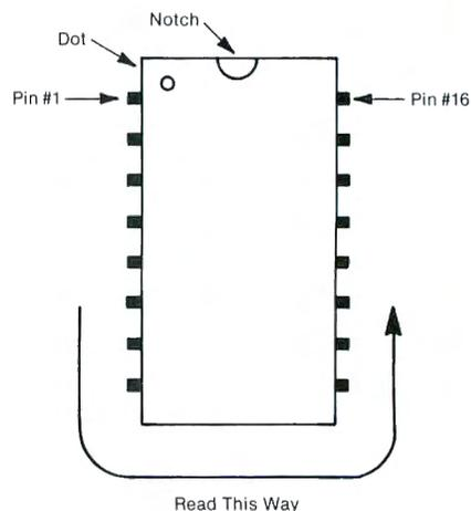
Fig. 2. How to read integrated-circuit pin numbers.
