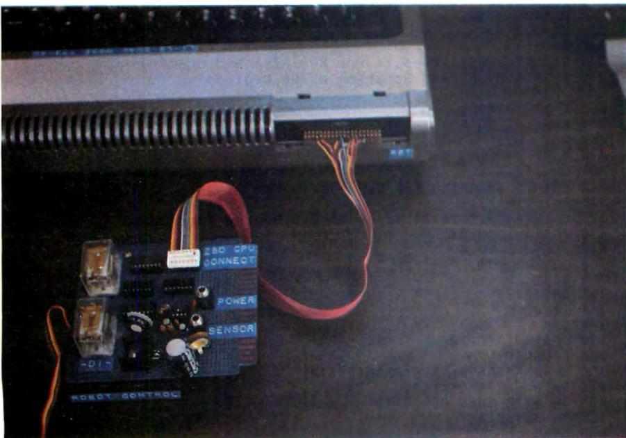
Photo 2. Interface control board connects to the TRS-80 by means of a 40-pin edge connector. Note the 14-pin DIP connector at the other end of the rainbow cable.
