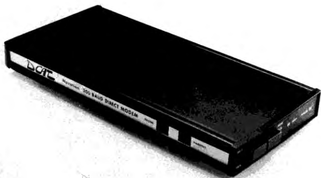
Photo 2. This is the DCAT. It is the direct connection version of the popular Cat modem. Direct connection means the modem plugs into the phone jack and does not use acoustical coupling. The Cat and DCAT require an RS-232 interface to the computer.
