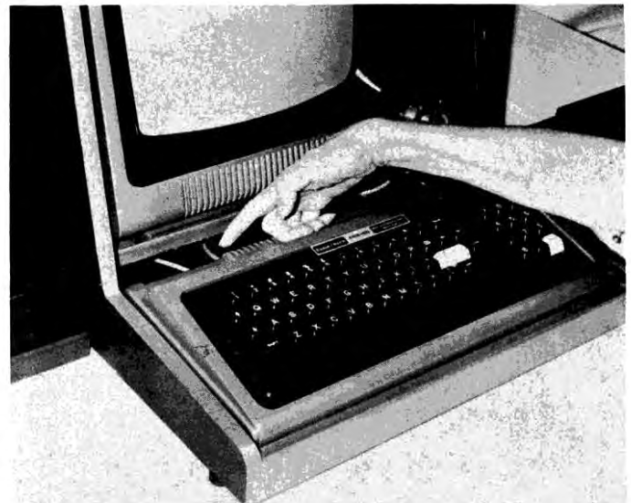
Photo 3. Make sure you can reach the on/off and reset switch.
