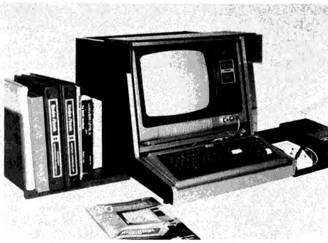
Photo 1. The complete system, up and running: Note the hood to eliminate glare and feet on each corner to give a free flow of air for cooling.
