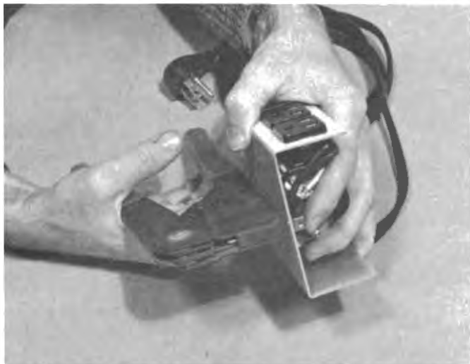
Photo 9. Fasten brackets to chassis. These will be used to hold the top cover in place. (Photos continue on next page.)
