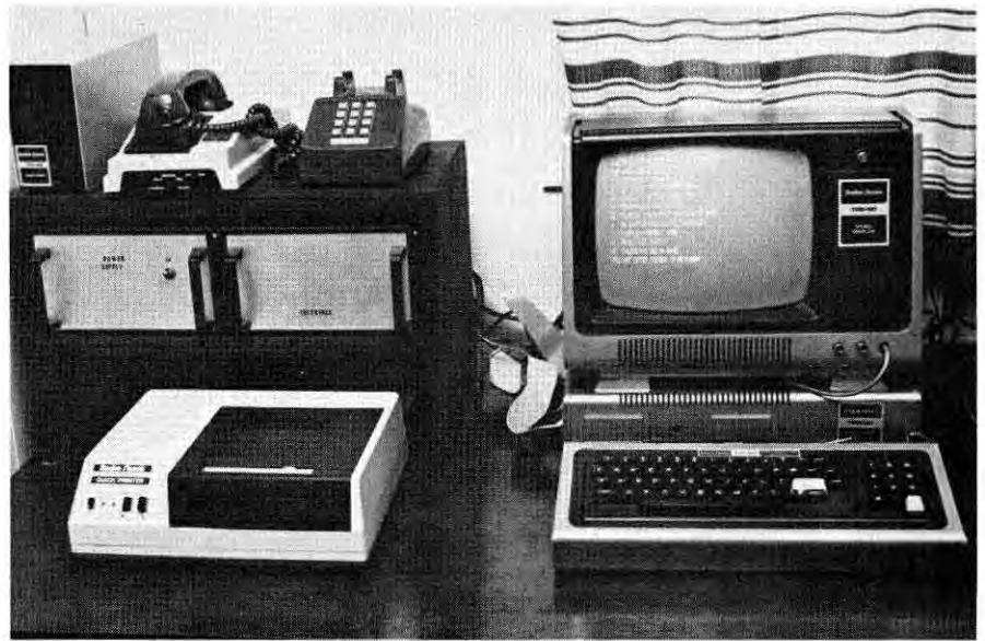
Photo 3. The "brain" of the Fairborn Observatory is an unattended TRS-80 and small six-chip interface designed by the author. Once the program is loaded, the video monitor is turned off and control is maintained from the telescope, some 60 feet away.
