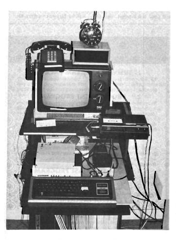
The author's system. The TV is driven by an RF modulator enclosed in the case that contains the Electronic Systems TRS-80 I/O board and power supply. This case is located just behind the keyboard on top of the A 103 modem. TRS-80 Serial I/O Board Electronic Systems San Jose, CA \$79.95 assembled \$59.95 kit
