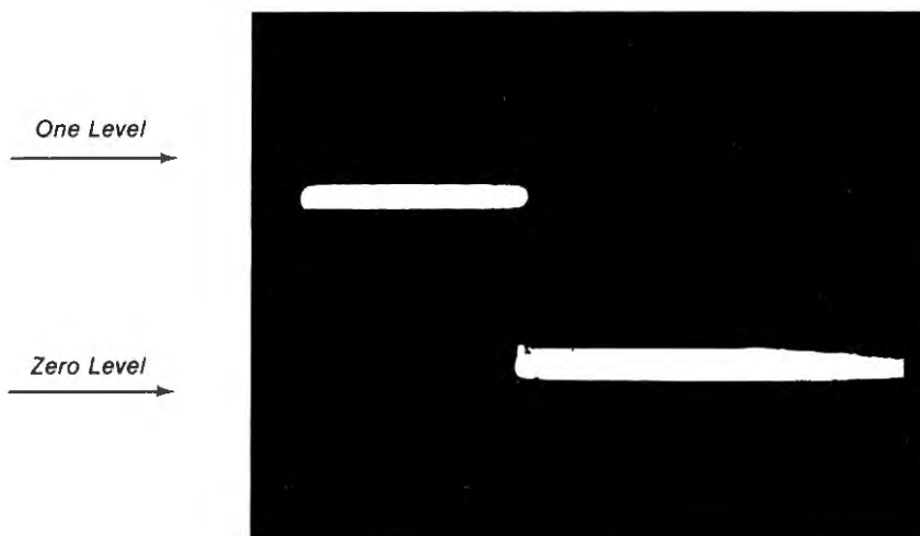
Photo 1. CSAVE signal measured before audio processing. Note that change from one-level to zero-level is invisible.
