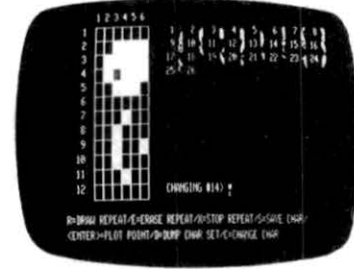
CHARACTER GENERATOR The supplied character generator software allows you to create your own character set of up to 64 original characters.
