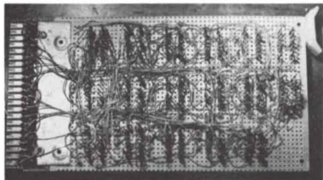
Photo 4 and Photo 5. The driver circuit board. Wire wrap sockets and a slit-n-wrap tool were used. The 44-pin edge connector is for use in a home made card cage.
