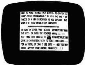
INVERSE VIDEO The 80-GRAFIX board allows you to do inverse video to high-light your screen displays.
