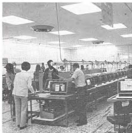
Finished units are then put into a further burn-in test.
