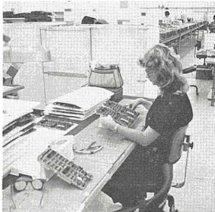
Once stuffed, the boards are inspected to make sure all the parts are there... and in the right place.
