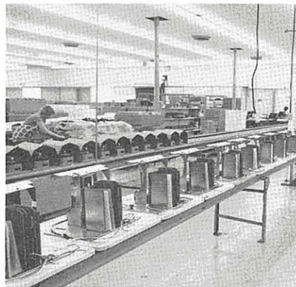
The system now starts getting put together. The monitor units, at the left, have been unpacked and inspected. They are covered to prevent damage.
