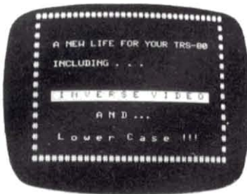
LOWER CASE The 80-GRAFIX board includes two sets of lower case characters at no additional cost.
