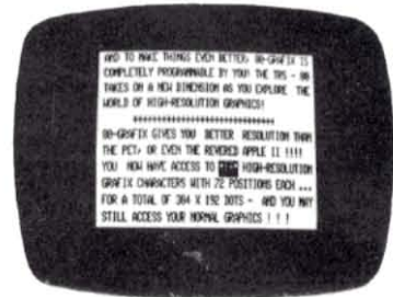
INVERSE VIDEO The 80-GRAFIX board allows you to do inverse video to high-light your screen displays.
