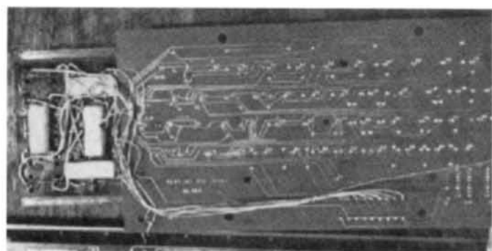
Photo 2. Wires run from points on the main keyboard's p.c. card directly to hex keypad. White rectangles are plastic foam that helps cushion the author's abusive typing style.
