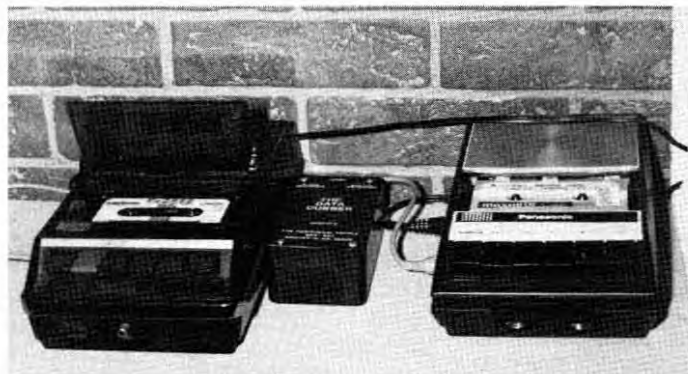
Duplicating tapes is easy with this setup. Pulses from the right cassette are regenerated by the Data Dubber. These replicas of the TRS-80 CSAVE pulses are recorded by the left cassette.
