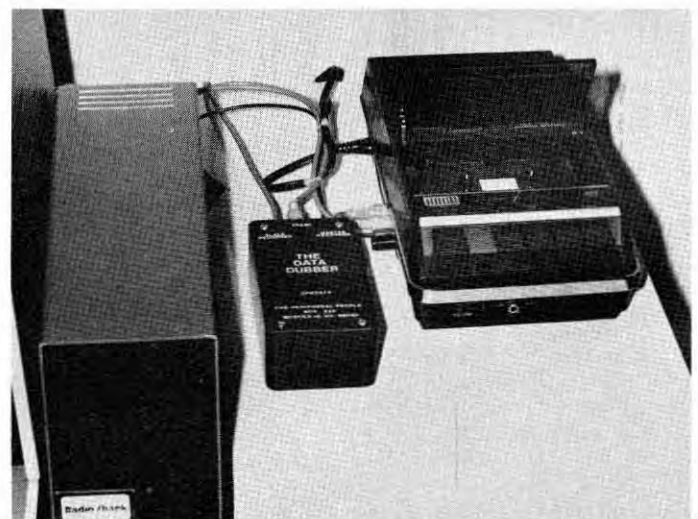
The Data Dubber can be connected in line between the cassette recorder and the TRS-80 CLOAD input.
