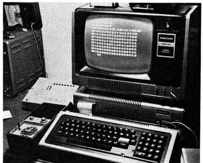
Photo 2. The author's system with newly installed hexadecimal keyboard and an AM radio.
