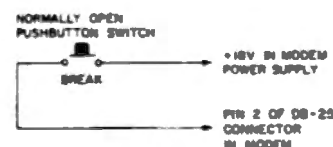
Fig. 1. Adding a BREAK key on to the modem.
