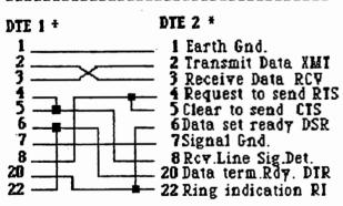
\*DTE= Data Terminal Equipment DCE= Data Communications Equip.
