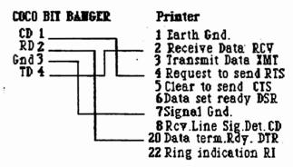
Coco Bit Banger Port RS-232 Printer Cable
