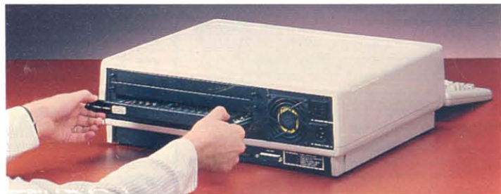
You can slide expansion boards easily into slots in the back of the computer (as shown above).
