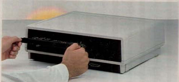
You can slide expansion boards easily into slots in the back of the computer (as shown above).
