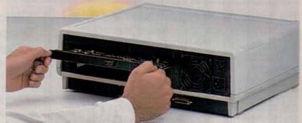
You can slide expansion boards easily into slots in the back of the computer (as shown above).
