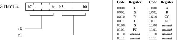
If an invalid register encoding is used for the source, a constant value of FF<sub>16</sub> or FFFF<sub>16</sub> is transferred to the destination. If an invalid register encoding is used for the destination, then the instruction will have no effect. The invalid register encodings have valid meanings when executed on 6309 processors, and should be avoided in code that needs to work the same way on both CPU's.
