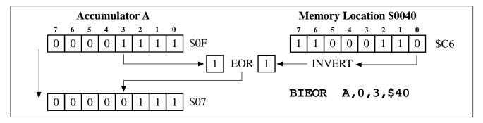
The figure above shows an example of the BIEOR instruction where bit 3 of Accumulator A is Exclusively ORed with the inverted value of bit 0 from the byte in memory at address 0040 (DP = 0).
