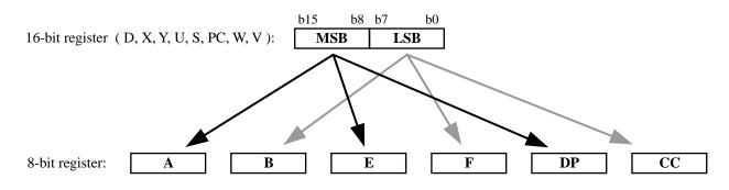
The EXG instruction requires a postbyte in which the two registers that are involved are encoded into the upper and lower nibbles.
