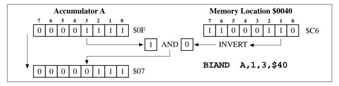
The figure above shows an example of the BIAND instruction where bit 3 of Accumulator A is ANDed with the inverted value of bit 1 from the byte in memory at address 0040 (DP = 0).
