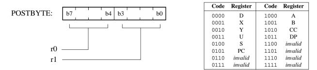
If an invalid register encoding is specified for either register, a constant value of  $FF_{16}$  or  $FFFF_{16}$  is used for the exchange. The invalid register encodings have valid meanings on 6309 processors, and should be avoided in code intended to run on both CPU's.
