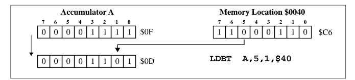
The figure above shows an example of the LDBT instruction where bit 1 of Accumulator A is Loaded with bit 5 of the byte in memory at address 0040 (DP = 0).
