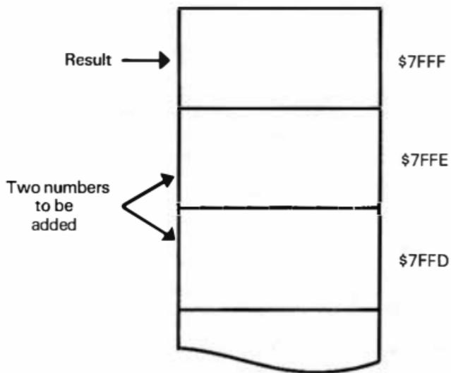
**Fig 3.1 Data for simple addition**
