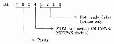
If the parity value is 000, then parity = none If the parity value is 101, then parity = MARK, no check If the parity value is 111, then parity = SPACE, no check
