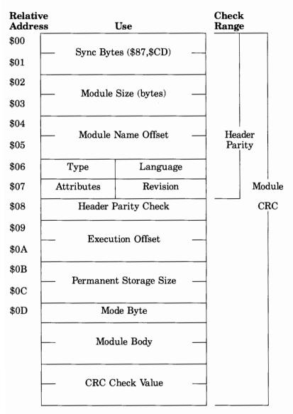
\$0D Mode Byte - (D S PE PW PR E W R)
