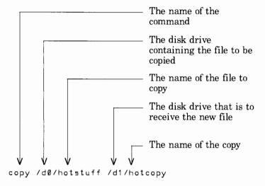
This command line tells OS-9 to copy a file named Hotstuff from your floppy disk Drive /D0 to a second floppy Drive /D1. The file copy is given the new name, Hotcopy.
