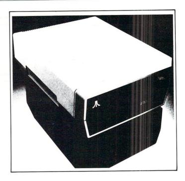
To load the DOS, the 810 disk is turned on and the Master Diskette (containing the DOS) is inserted. The Atari computer itself is then turned on, which automatically drags the DOS into memory. After about ten seconds the message "READY" appears on the screen. Now, when you type the command "DOS", a menu will appear:
