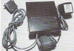
CmC's ADA 1400 drives a printer with an RS-232 interface from the Commodore PET IEEE-488 bus. The ADA 1400 is addressable, works with the Commodore disk and prints upper and lower case ASCII.
