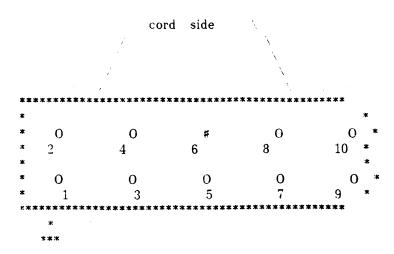
Monitor Jack Pin PinOut Def.
