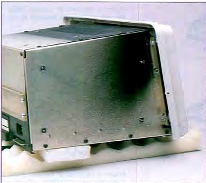
Photo 3. The left side of the 4P, showing the screws holding the main PC board in the pan.
