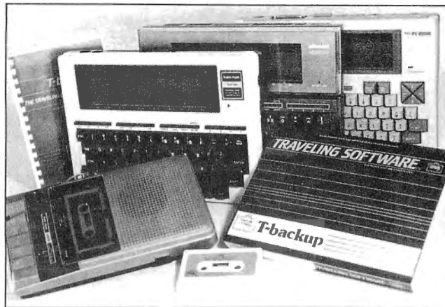
T-Backup backs up Model 100 memory in four minutes.
